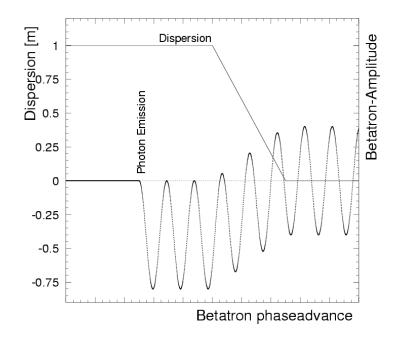
An ideal, flat accelerator has only horizontal dispersion, i.e. extremely small vertical emittance. In real machine, coupling and spurious vertical dispersion increase vertical emittance.
