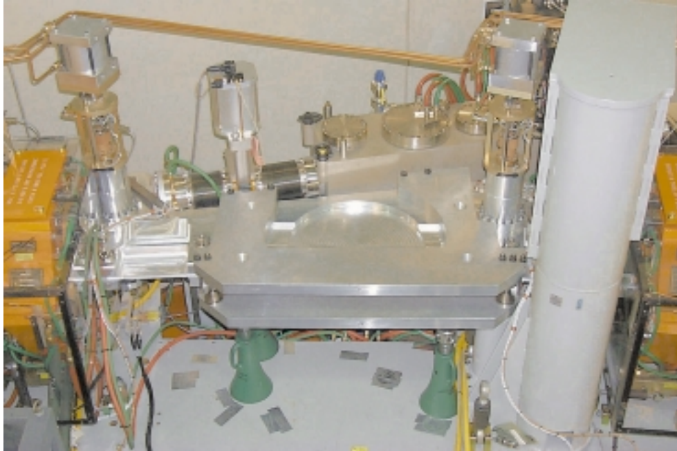
Figure 8 One of the three ALS vacuum chambers after machining in situ to prepare for superconducting bend magnet installation.
