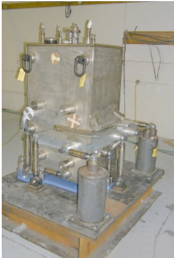
Figure 7 The first superbend magnet cryostat system.
