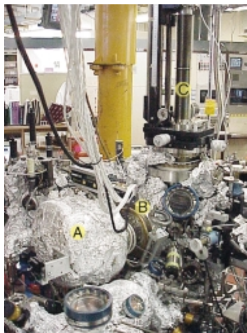
Figure 4 The upgraded high-resolution photoemission chamber on Beamline 7.0.1: (A) new SES-100 imaging spectrometer with (B) differentially pumped rotary seal around its lens; (C) new liquid-helium cryostat and goniometer.
