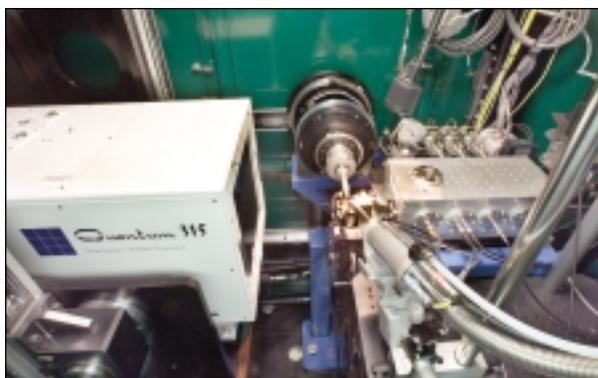
**Figure 6** The inside of the Beamline 8.2.2 hutch, showing the x-ray detector (*left*) and the single-axis air-bearing rotation stage (*center*).
