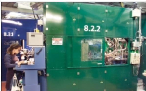
**Figure 5** Minihutch endstations in Sector 8. The back panel of the Beamline 8.2.1 minihutch is visible to the far right.
