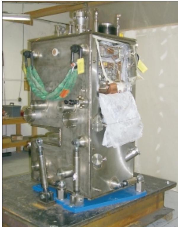
**Figure 2** First ALS superbend magnet produced by Wang NMR.
