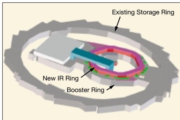
**Figure 6** The infrared ring location atop the ALS booster synchrotron. The ring circumference is 66 meters.
