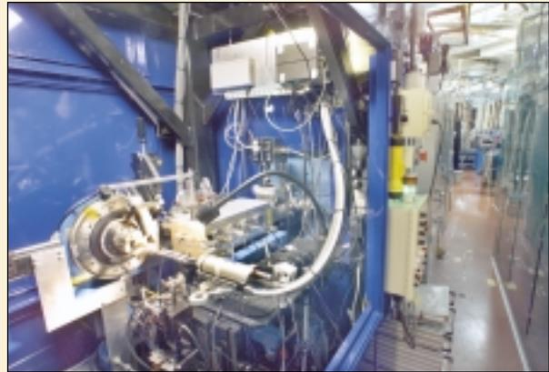
Beamline 8.3.1, the first beamline to accept light from a superbend magnet at the ALS.
