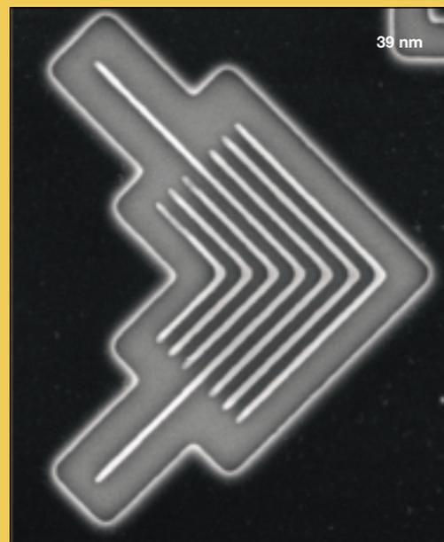
**Figure 2** Modifying the exposure process can decrease the minimum feature size for some types of patterns. Here, by overexposing an elbow test pattern with the lines somewhat farther apart than in the pattern with equal line widths and spacing imaged in Figure 1, the CXRO team was able to print line widths down to 39 nm with the ETS Set-2 Optic.
