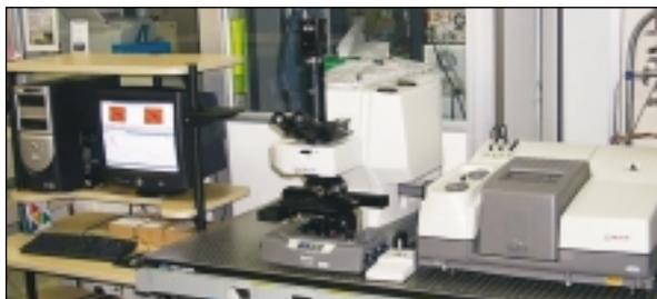
**Figure 3** The new infinity-corrected infrared microscope on Beamline 1.4.3.
