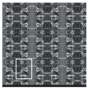
The momentum-space distribution of electronic states at the Fermi level determined in the present study. The raw data (rectangle) are tiled to highlight the square lattice arrangement of the features.
