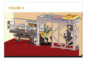
Layout of the SIBYLS beamline, showing the upstream SAXS station *(left)* and the downstream PX station *(right).*
