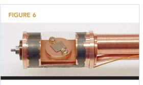
New cryogenic sample holder used for the experiments.
