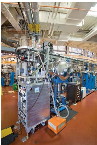
FIGURE 1 Mini Magnet endstation installed at bending-magnet Beamline 6.3.1.
