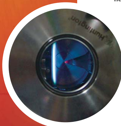
FIGURE 1 Right: The low-pressure flame apparatus in operation at the ALS. The luminous zone of the flame is visible as the bright blue line on the left. The tip of the quartz sampling cone is glowing red. The burner can be moved horizontally to place the sampling tip at any point in the flame. Photograph by Daniel Strong, courtesy of Sandia National Laboratories.
