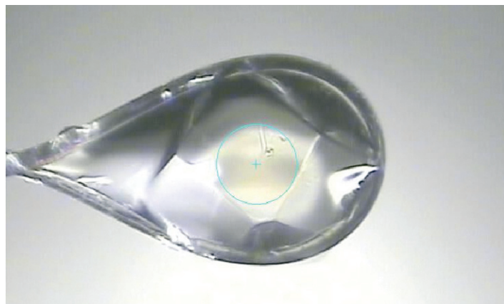
Sample viewing using the MD2 microdiffractometer at Beamline 8.2.1; circle is 100 microns in diameter.
