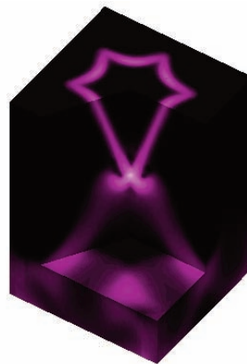
Three-dimensional image of the surface band structure of bismuth telluride ( \text{Bi}_2\text{Te}_3 ). The V-shaped pure surface state is nearly isotropic in the momentum plane, forming a Dirac cone in momentum space. (Image courtesy of Yulin Chen and Z.-X. Shen, Stanford University.)
