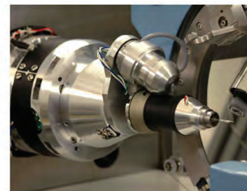
Sample viewing at Beamline 5.0.2 is in-line with the x-ray beam. In conjunction with a highly stable goniometer, MiniKappa stage, and CVC, this allows centering and data collection from crystals down to 5 microns in diameter.
