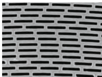
Free-standing EUV zone plate with pseudo-random support structures for minimized impact on imaging and optimal robustness.
