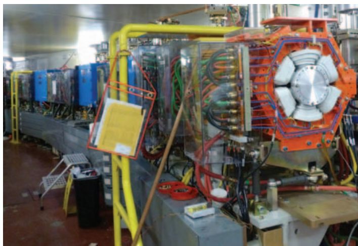
One of 48 new sextupole magnets installed in the ALS lattice as part of a major brightness upgrade.
