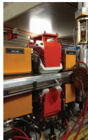
Left: New storage-ring bend-magnet supply, operational since March 2013. Right: One of 48 new sextupole magnets installed in the storage ring as part of the brightness upgrade.
