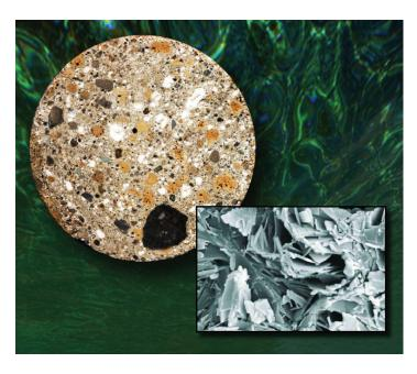
Drill core of mortar consisting of volcanic ash and hydrated lime, showing yellowish particles of pumice, dark gray fragments of lava, and white particles of relict lime (sample from M. Jackson and the ROMACONS research team). The light gray is the cementitious matrix that binds the concrete. Inset is a scanning electron microscope image of the special Al-tobermorite crystals that are key to the superior quality of Roman seawater concrete.
