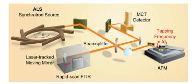
The experimental setup for SINS includes the ALS light source, an atomic force microscope, a rapid-scan Fourier transform infrared spectrometer, a beamsplitter, mirrors, and a detector.
