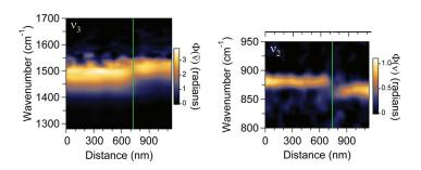
A spectral linescan of a blue mussel shell, which transitions from calcite to aragonite, illustrates the spatial resolution and spectroscopic range capabilities of the SINS technique. The image shows two simultaneously acquired vibrational modes across the transition region.
