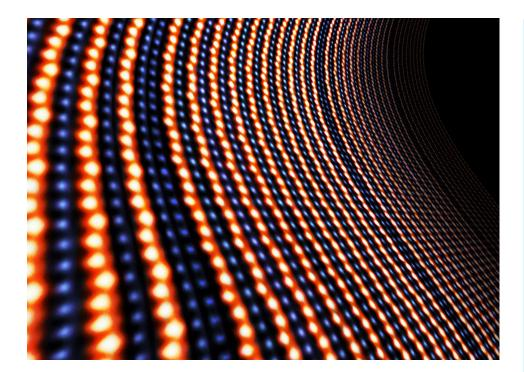
Scientists engineered a new magnetic ferroelectric at the atomic scale. A false-colored electron microscopy image shows alternating lutetium (yellow) and iron (blue) atomic planes. An extra plane of iron atoms was inserted every ten repeats, substantially changing the magnetic properties. (Credit: Emily Ryan and Megan Holtz/Cornell)
