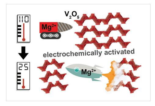
At high temperature (110 °C), magnesium ions (Mg<sup>2+</sup>) have enough kinetic energy to drill into an electrode made of vanadium oxide ( $V_2O_5$ ). The process breaks down the  $V_2O_5$  into smaller particles, which facilitates exit and subsequent reentry by magnesium ions at room temperature (25 °C).
