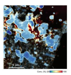
X-ray microscopy shows where magnesium was detected (red areas) in battery-electrode particles (vanadium oxide), when discharged (left) and charged (right). An effective electrode material accepts "guest" particles such as magnesium ions as the battery discharges and releases them during charging.
