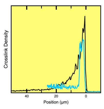
Crosslink density across the shells from the outer surface (position 0) to interior of SAP beads treated in two different ways. Comparison shows strikingly different profiles that reflect the complicated kinetics of the SAP swelling when exposed to liquid and the different shell-formation processes.
