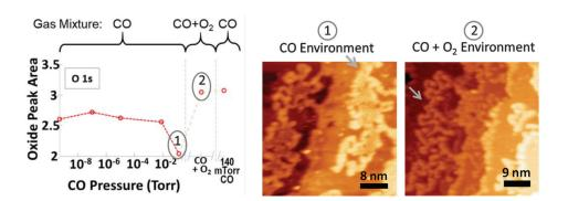
On surfaces containing oxygen vacancies, forming  $CO_2$  from CO consumes the oxide. When oxygen is added to the gas-phase sample environment in a 1:2 ratio with CO, the oxygen vacancies become filled and the surface is deactivated for the reaction. Combining the ALS results with HPSTM showed that the deactivation of oxide sites was accompanied by a transformation in the oxide structure.
