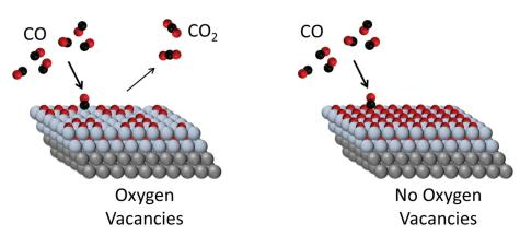
On metal-oxide catalyst surfaces with oxygen vacancies, CO is readily converted to  $CO_2$ . When the oxygen vacancies become filled, the surface is deactivated for the reaction. Gray = metal (platinum); blue = oxide (cobalt oxide); red = oxygen; black = carbon.
