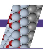
structures observed with HPSTM indicated that the stable carbonate is formed preferentially at the edges of CoO islands, where both Pt and CoO were exposed. Edge sites are often considered to be active sites, but for this catalyst, that's not the case.
