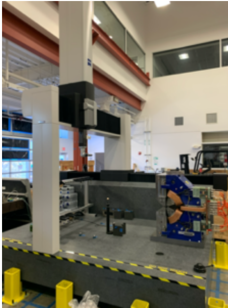
The new coordinate measuring machine in the ALS-U project's Magnet Measurement Facility. The device will take precise measurements of the new accumulator magnets and prototype storage ring magnets prior to mounting and aligning them in preparation to be installed. The blue magnet shown is a prototype magnet for the storage ring. (Credit: Steve Virostek/Berkeley Lab)
