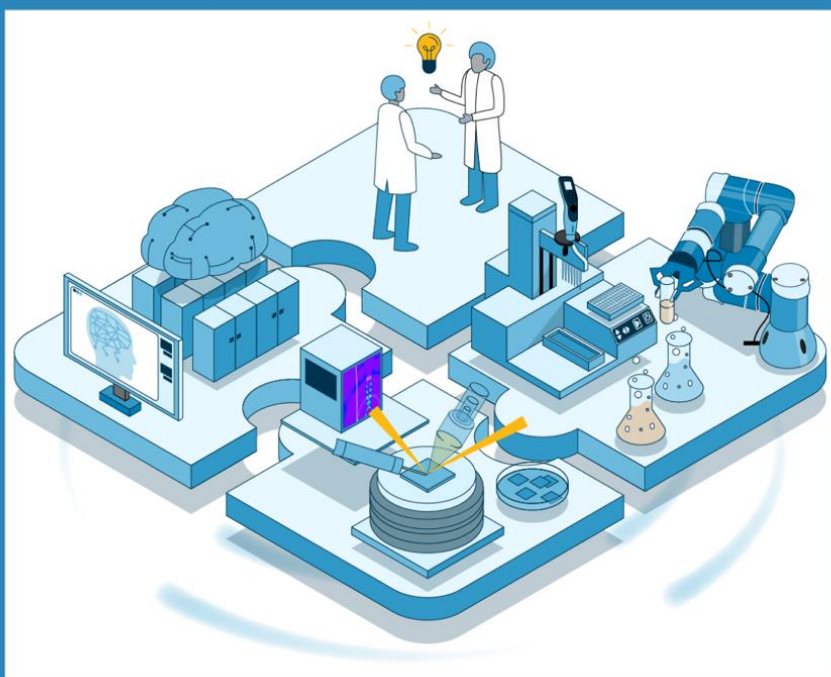
Fig. 8. Scientists (back) can use AI-assisted autonomous experiments to quickly discover and understand complex new materials by combining ALS multimodal in situ x-ray experiments (front) with robotic sample synthesis and handling (right) and advanced controls combined with high-performance computing (left).
