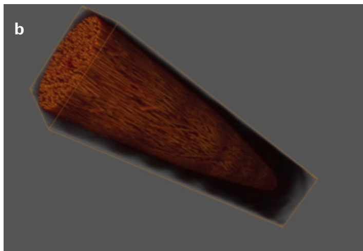
This 3D volume rendition of engineered polymer reinforced with glass fiber shows a (a) virtual cross-section and a (b) 3D image that illustrates the alignment of recycled fragments and virgin fibers in a narrowing injection-molded part. Individual fibers are 3µm in diameter.
