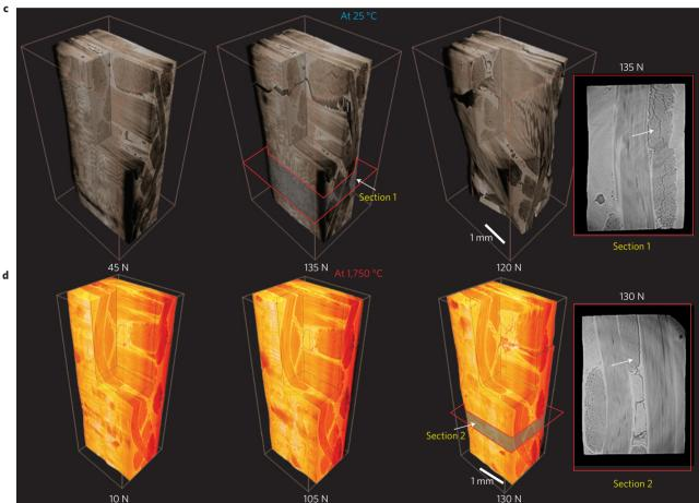
Figure 4 | In situ tomography of C-SiC composite with textile-based carbon fibre reinforcements under a tensile load at 25 and 1,750 °C.
