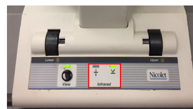
Figure 3: When the measurement mode changes, the appropriate green LED will illuminate on the microscope. In this image, the system is configured for viewing the sample in Reflection.
