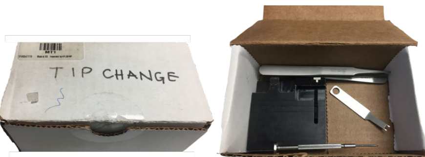
FIGURE 24. TIP CHANGE BOX. THIS BOX CONTAINS THE TOOLS NECESSARY FOR A TIP CHANGE. PLEASE RETURN ALL TOOLS TO THIS BOX WHEN TIP CHANGE IS COMPLETE.
