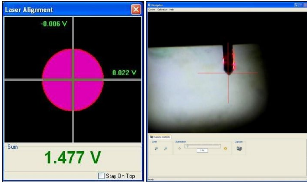
FIGURE 11. DEFLECTION LASER ALIGNMENT. LEFT: POSITION SENSITIVE DETECTOR (PSD) FOUR QUADRANT SIGNAL IN THE LASER ALIGNMENT WINDOW. RIGHT: OPTICAL MICROSCOPE IMAGE OF CANTILEVER IN THE NAVIGATOR WINDOW.
