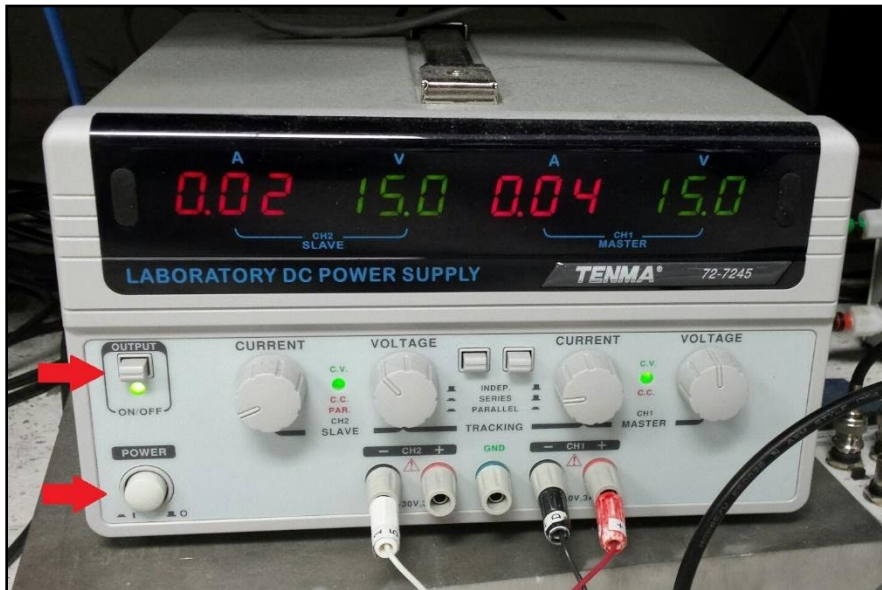
FIGURE 5. POWER SUPPLY FOR THE MCT DETECTOR. THE SUPPLY AUTOMATICALLY RECALLS THE APPROPRIATE SETTINGS: TURN ON THE POWER WITH THE LOWER BUTTON (INDICATED BY LOWER RED ARROW), THEN ENABLE THE OUTPUT BY PUSHING THE BUTTON ON THE UPPER LEFT (UPPER RED ARROW).
