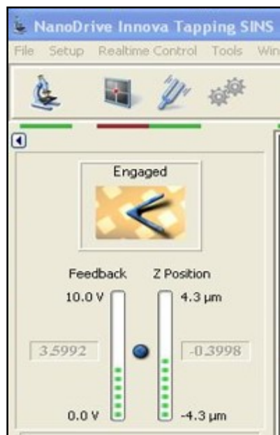
FIGURE 15. SETPOINT AND FEEDBACK CONTROL. THE UPPER-LEFT OF THE NANODRIVE WINDOW HAS ACTIVE FEEDBACK AND Z POSITION MONITORS.
